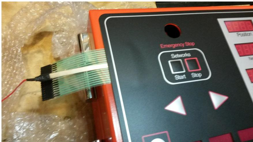
4. Position the membrane so all displays are viewable through the red transparent windows, the hole for the emergency stop button is correctly aligned and the status LED's are viewable through the 5mm square clear windows.
