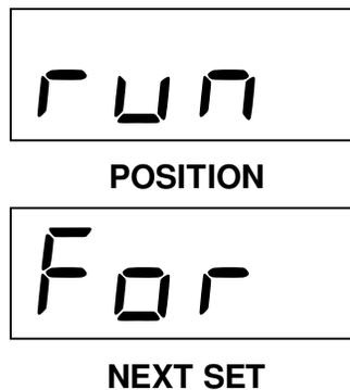
After the “C” function has been selected, the displays in the centre of the console will appear as shown above. The operator will then press Enter to initiate the function. The drive signal will then be applied to the forward valve until the Clear button is pressed.
