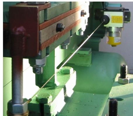
**Important:** Additional steps are required when calibrating a machine that uses a rotary encoder with spring return wire rope mechanism. Please refer to the additional details in 'Note2' later in this section.
