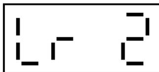
When a random pushbutton is pressed, this display will show the value of the random number entered. If this number is then programmed to a pre-programmed pushbutton this random number disappears and the Layer number will return. If the “Enter” pushbutton is pressed this random number will shift up to the Next Set, or onto the stack, and the layer number will return.
