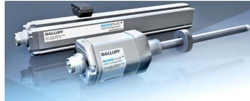
These devices give approximately 22-23 raw counts/mm travel, and raw counts increase as the magnet moves away from the end with the electrical connector (usually as cylinders extend or machines move forward). Where a networks has been configured for using a transducer the 'Probe Type' parameter (P120/220) will be set to '1' for a start/stop pulse type (most common), '2' for a PWM or L type, and '3' for an SSI type.
