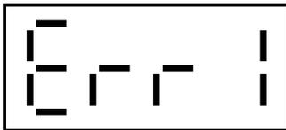
This message is shown when the operator has entered the incorrect PIN number to enter either Function or Parameter Mode. The message will be displayed in the Layer display for approximately 2 seconds.
